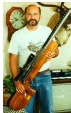
John is shown with his Remington model 721 action and a walnut laminated stock he made. The barrel is a Hart stainless steel match barrel. The scope is a Leupold 24X target scope. the rifle is chambered for a .30 Cal. cartridge which he designed based on the 8mm Rem. Mag. Cartridges were loaded using Federal 215M primers, IMR 7828 powder, and of course the Sierra 200 gr. HPBT MatchKing bullets.
