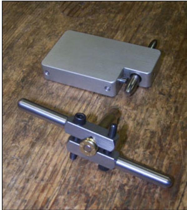
Our main goal in outside neck turning is to give our seating die it's best chance to seat a bullet with good concentricity with as little of run out as possible. This puts our bullet in better alignment with the center of the case body and in a squared and trued action, more perfect alignment with the bore.
